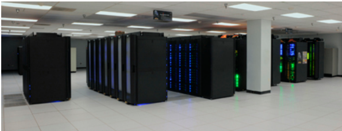
NCCS recently doubled the capacity of its Discover supercomputer by adding a Dell PowerEdge C6100 cluster with 1,200 Westmere nodes (left). Discover now has a combined 2,864 nodes (29,368 cores). Photo by Pat Izzo, NASA Goddard Space Flight Center.
